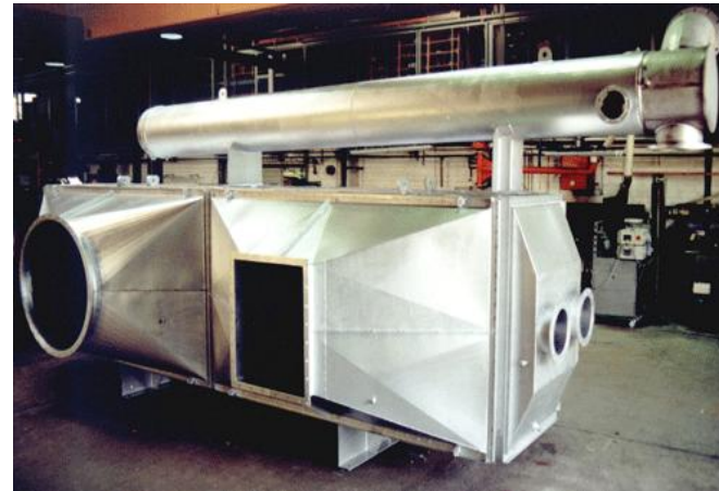
Housing for heat exchangers, made of highly heat-resistant stainless steel
